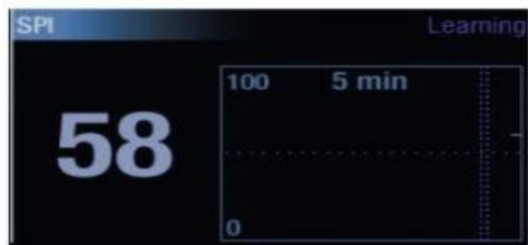
SPI learning at the beginning of the operation. The number is displayed in grey.
